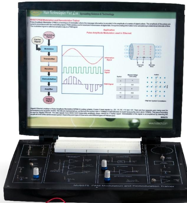
**Nvis 6575 PAM Modulation and Demodulation Trainer** is a useful training product for the students to help them understand the concept of Modulation and Demodulation. Pulse Amplitude Modulation is an effective technique used to transmit the information signal over a long distance without any distortion in it.
